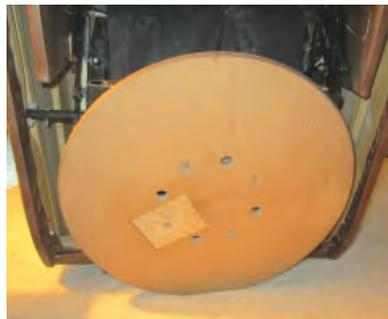
a look and found one of four mounting bolts had pulled most of the way through the composite disc. I unbolted the disc, cut out the five-inch square of broken material, glued in a piece of 3/4 inch plywood, drilled a counter-sink hole along with an attaching hole and reassembled it. It's been a successful fix, so far.
