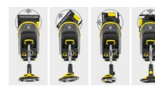
The roller brush head of the new BR 35/12 C Bp is an outstanding technical innovation: It can be horizontally rotated 200° in both directions around the steering axle. This means that every part of the full circle is covered, finally eliminating blind spots when cleaning. In the parking position, all pressure is taken off the brushes to prevent any damage.
